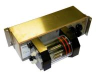
The model I8050-7 Sensor Module comes complete with two thermometers. The first is fitted near the water sampling port to accurately measure the temperature of the surface waters, while the second is fitted inside the measuring cell to allow salinity calculations.
