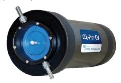
The  $CO_2$ -Pro<sup>TM</sup> CV measures the partial pressure of  $CO_2$  gas dissolved in water using infrared detection. Standard ranges from 0-600 ppm up to 0-10,000 ppm, as well as custom ranges, are available that cover the full spectrum of pCO<sub>2</sub> needed for accurate measurement of ocean, coastal, riverine, and lake  $CO_2$  levels.
