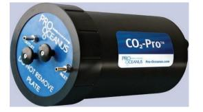
The  $CO_2$ -Pro instrument measures the partial pressure of  $CO_2$  gas dissolved in water using infrared detection. Standard ranges from 0-600 ppm up to 0-2000 ppm provide the full spectrum of p $CO_2$  required for accurate measurement of ocean  $CO_2$ .
