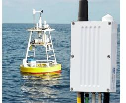
DANTE has the connectivity to integrate a large suite of instruments, and supports virtually any oceanographic or environmental sensor in use today. The uniquely modular controller design makes a DANTE monitoring system extremely expandable and configurable. Each buoy controller can be customized by selecting modules to suit the sensor interface requirements. Future requirements can be met with new types of plug-in modules offering an inexpensive and flexible way to add new capabilities.
