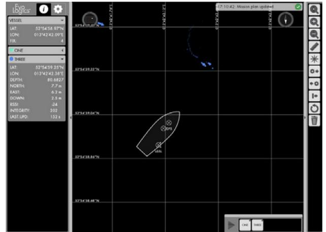
Evologics SiNAPS is a client-server application. The SiNAPS server is a software component, installed on the Navigation computer interfaced with the USBL transceiver and other external instruments. The SiNAPS server receives, processes and stores data from the USBL transceiver and external instruments. It performs all the necessary calculations to display this information on-screen.
