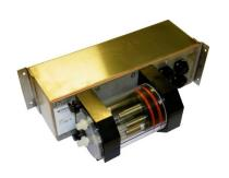
The model I8050-7 Sensor Module comes complete with two thermometers. The first is fitted near the water sampling port to accurately measure the temperature of the surface waters, while the second is fitted inside the measuring cell to allow salinity calculations.
