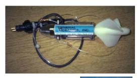
The model 2135 is a real-time readout, hand held microprocessor controlled data acquisition unit. When used in conjunction with our flowmeter sensor, this battery operated waterproof unit displays current velocity in cm/sec, ft/sec. m/sec, or knots. The easy-to-read two line liquid crystal display also gives you total distance travelled. The microprocessor based unit provides an event timer with external start/stop freeze display switch.
