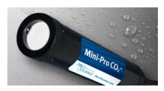
The Mini-Pro  $CO_2$  uses infrared detection to measure the partial pressure of  $CO_2$  gas dissolved in liquids. With pC02 ranges from 0-500 ppm up to 0-100%, the Mini-Pro C02 provides the versatility needed for any application.
