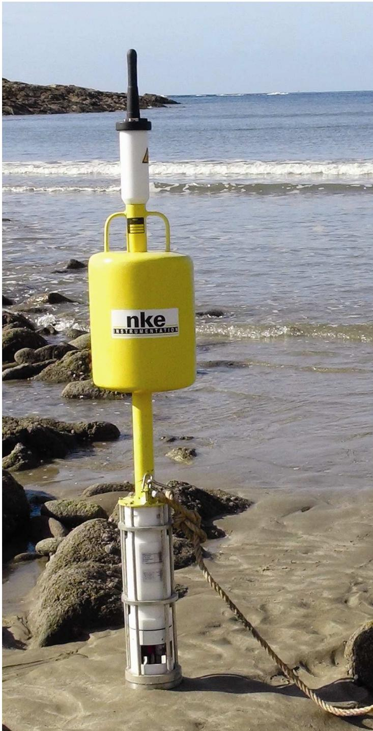
SMATCH measures and records up to 7 parameters: temperature, pressure (depth), conductivity (salinity), turbidity, dissolved oxygen, fluorescence (Chlorophyll a, Phycocyanine, Phycoerythrin) and pH. Light and compact, SMATCH has been designed for long term use in network.
