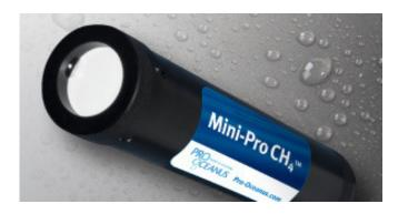
The Mini-Pro CH<sub>4</sub> instrument uses infrared detection to measure the partial pressure of CH<sub>4</sub> gas dissolved in liquids. Conversion to dissolved methane is simple with known temperature and salinity values.
